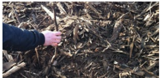
Figure 6. Hog fuel (pictured here) cannot be used in the combustion systems discussed in this guide.
