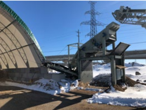
Figure 29. Wood chips are chipped with conventional, hand-fed chippers and then screened with a three-deck aggregate screener to filter out fine and coarse particles, leaving only chips of the appropriate size for the bioheat system. (Photo: Biothermic)
