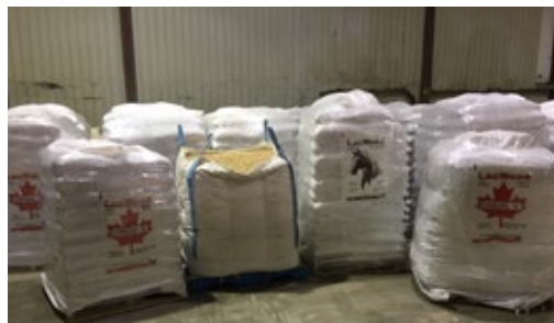
Figure 7. Pellets can be delivered in 18 kg bags on a wrapped pallet (left) or in large tote bags (right). (Photo: ICS Lacroix)
