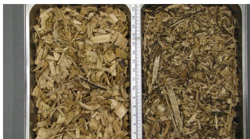
Figure 2. A high-quality wood chip (left) and a lower quality wood chip (right).
